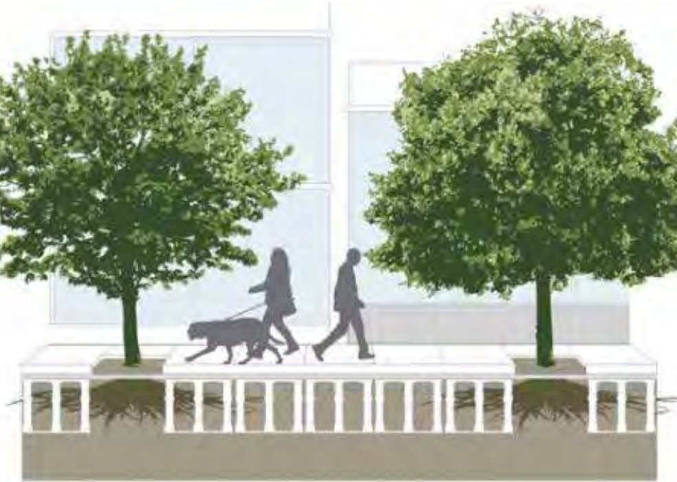
Figure 13.2.6 (b) Structural Cell Example
