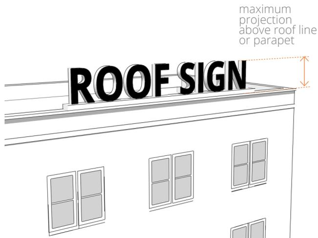
Figure 8.8-B Example of Roof Sign
