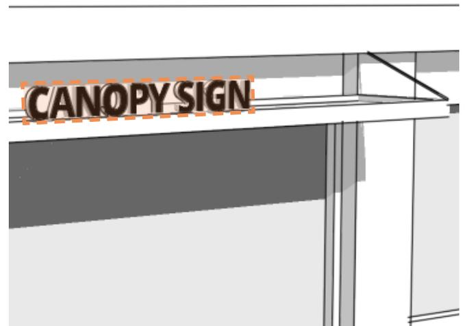
**Figure 8.7-C** Area Calculation for Canopy-Mounted Sign
